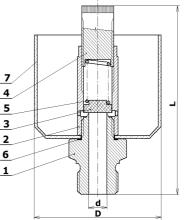
While in service these pressure regulators run nearly maintenance-free. In case the tapered plug remains closed for longer than 14 day it may get stuck to its valve seat. Therefore, once in two weeks carry out its functional test by lifting it with a thin rod without sharp edges, e.g. a little hook, or by sensitive loosening of the adjusting screw until inside overpressure opens the valve (slight fizzing noise or first bubbles in indication water).
